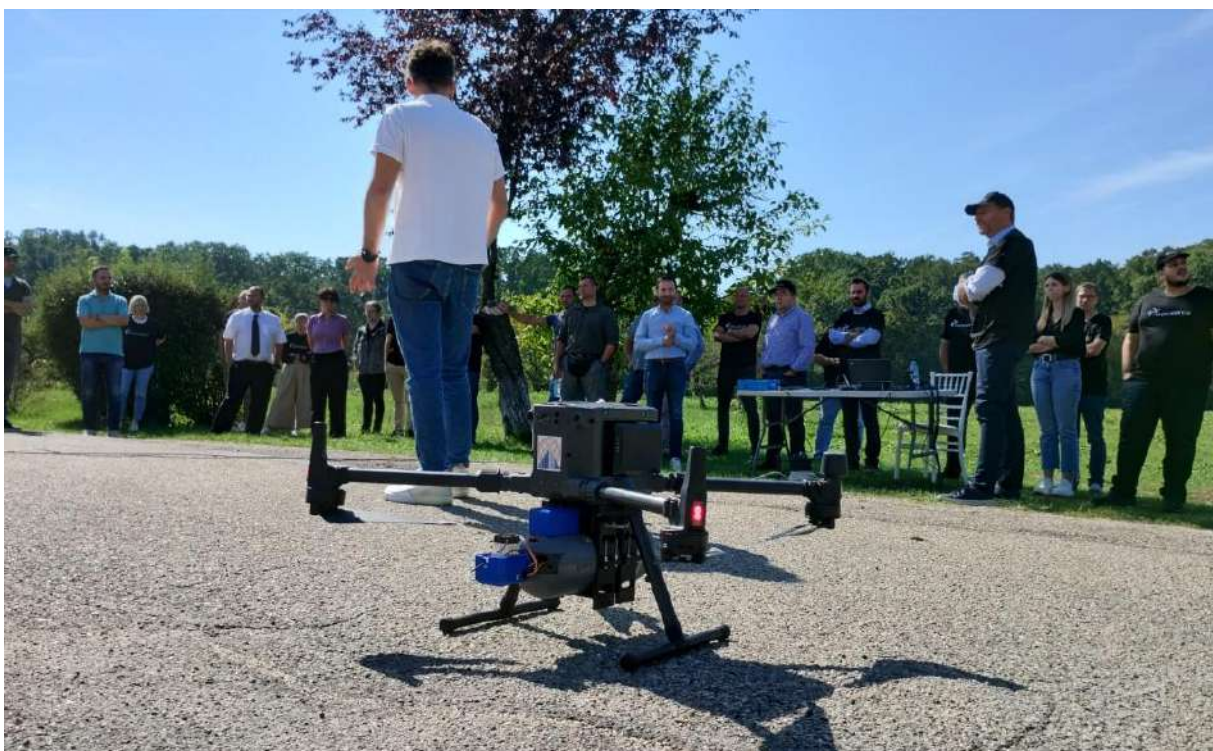
UAV carrying the T4i Dover Ultra detector (Photo: SPP)
