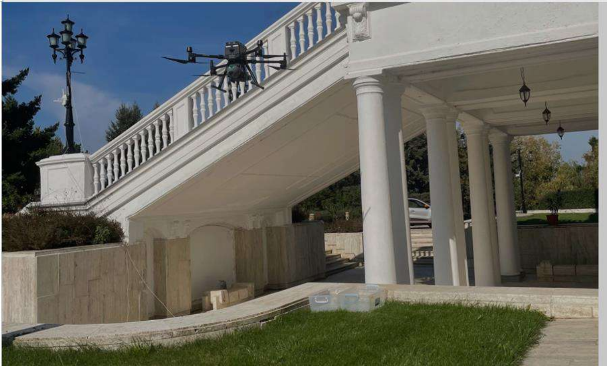
The UAV carrying the T4i Dover Ultra approaches the source of the explosive precursor on the ground (Photo: Stodiek)
