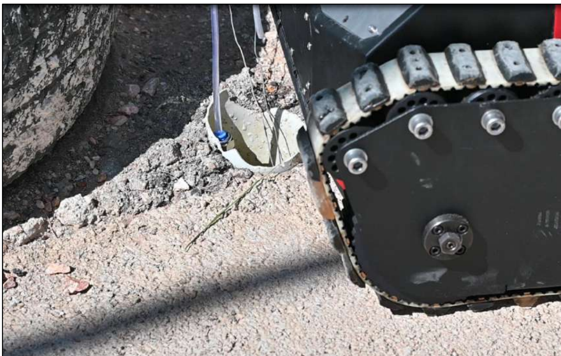
The UGV releases a pipe into a water whole below to take a sample from the liquid within (Photo: P. Vasilev)
