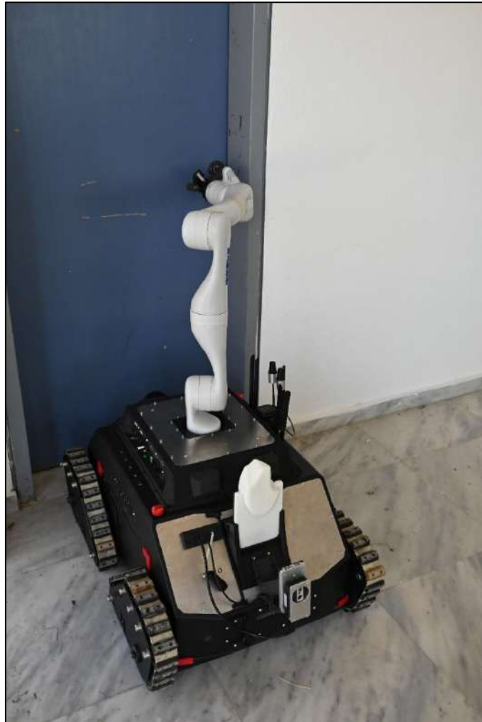
The UGV opens the door with its gripper on the arm (Photo: P. Vasilev)
