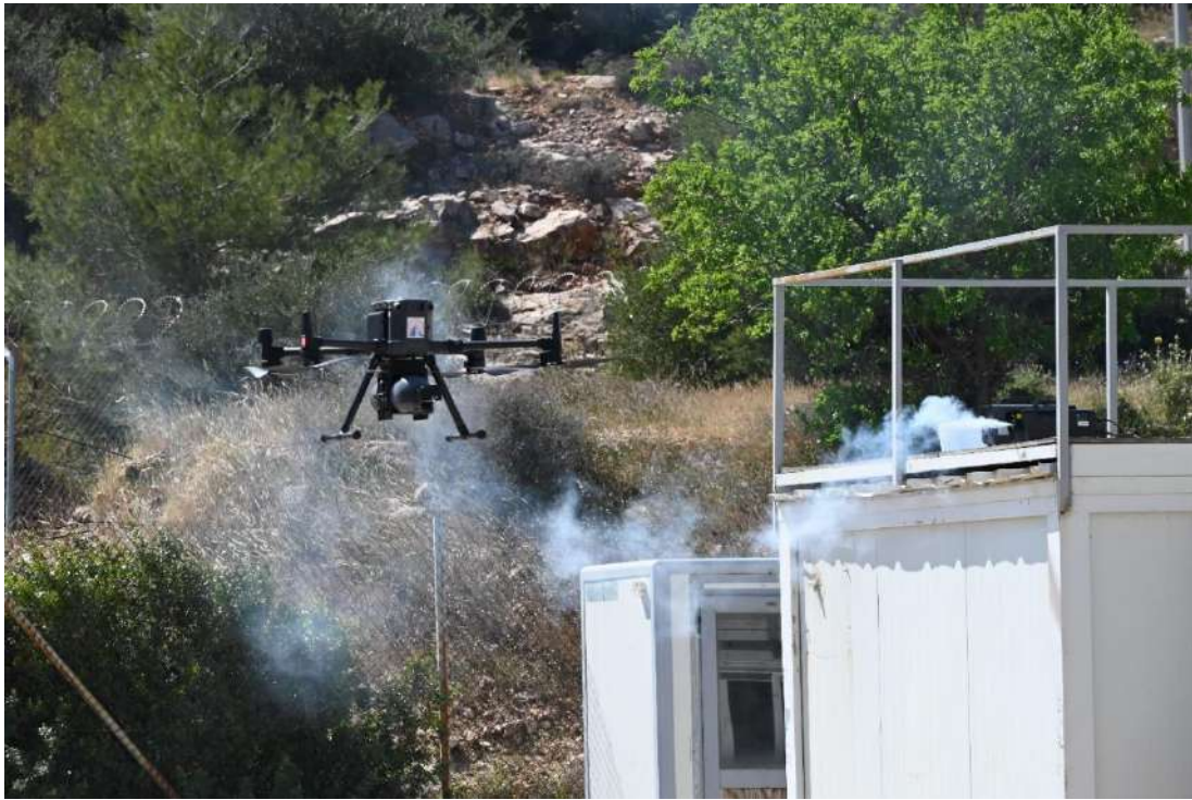
The UAV carrying the T4i Dover Ultra approaches the source of the explosive precursor (Photo: P. Vasilev)
