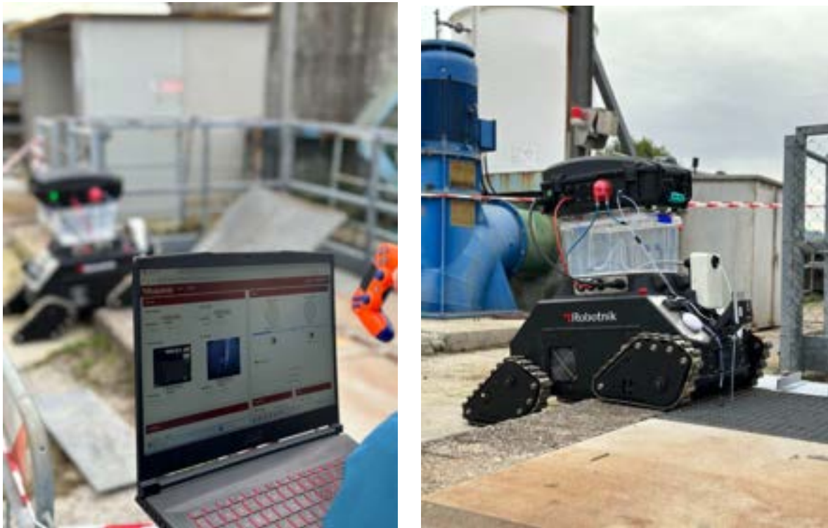
The teleoperated UGV is taking water probes (Photos: Robotnik)
