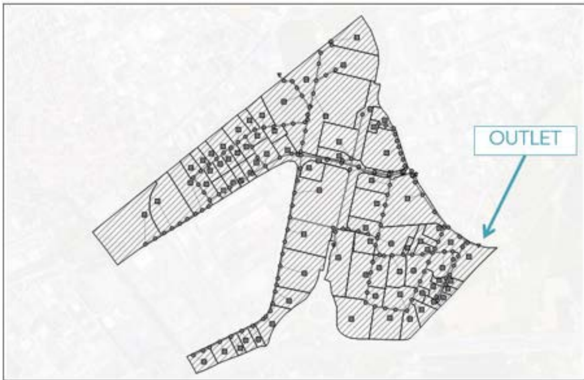
Figure 3: Map of an industrial zone indicating the locations of numerous inlets into the sewage system as well as the manholes installed for network inspection.
